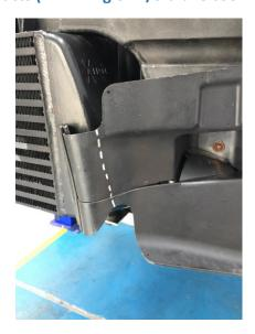
Remove the ambient air temp sensor bracket and bolt to modified crash bar with m5 x 16 socket head bolt and nylock supplied
