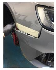
8. Unclip headlight washer pipe then remove bumper making sure to unclip parking sensor loom plug.
