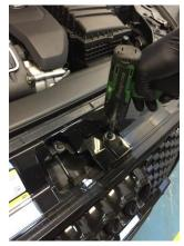
2. Undo headlights (NO NEED TO REMOVE) 3x T30 torx
