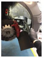
5. Undo 4x T20 torx holding fibre inner arch to gain access to bumper bolts
