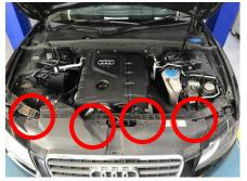
2. Undo 2x T25 securing top of bumper
