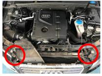
3. Undo 2x T25 torx securing inner arch to bumper
