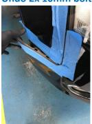
6. Remove bumper making sure to unclip fog lights. Store in a safe place to prevent damage
