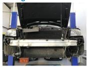
7. Remove standard cooler by removing boost pipes. Undo 1x T25 on passenger side and unclip cooler.
