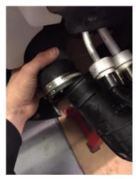
20. Install new Airtec intercooler using brackets supplied. Axle stands are advised to support the weight until brackets are in position and cradle re-attatched.
