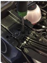
12. Unclip bonnet catch sensor clip x2 L/R from crash panel.
