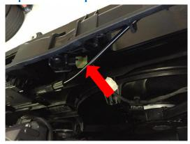
15.Unbolt 3 bonnet catches and slide out & lay across engine 6x 10mm bolts.
