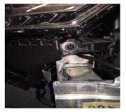
9. Unclip washer jet & air temp sensor and move to the side.
