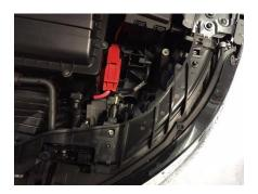
8. Remove 1x T30 torx below headlight to drop headlight washer cradle down.
