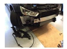
10. Remove 7x T30 from rad pack to slam panel, remove horns from O/S.
