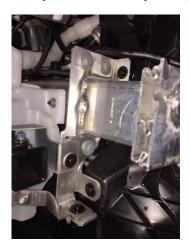
11. Remove 4x T27 from slam panel & top of engine bay.
