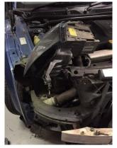
6. Remove both side mounts & lower boost pipe 3x13mm bolts on each side of boost pipe.
