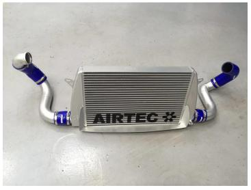
13. Install new Airtec intercooler into place, as per picture below
