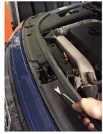
2. Remove under tray 14 torx, 2 screws, 2 screw in each arch
