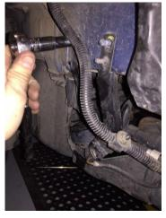
9. Unbolt & unclip air temp sensor from 1<sup>st</sup> cradle.
