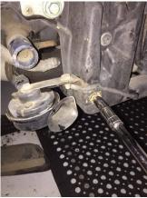
**11.**Put alloy spacer in bolt hole, slide new Airtec intercooler in from bottom and bolt up
