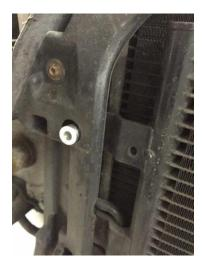
12.Horns need to be moved for new pipework. Brackets can be loose and adjusted then re-bolted to where standard side mount bolts into chassis rails.
