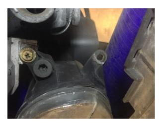
14. Also the bumper as shown below will also require cutting. If the bumper doesn't line up correctly you may need to remove more around this area, the fog light grilles normally fit without cutting, but have been known to require some small adjustments on some cars
