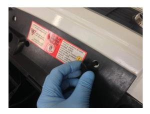
2. Remove the x 2 T20 Torx on each side of the inner wheel arches
