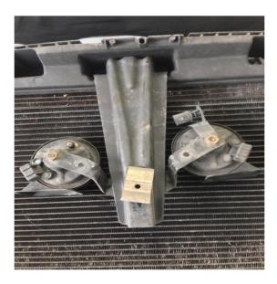
9. Modify horn bracket as shown below and secure horns with new brackets provided, the 3 bracket is for the Ambient air temp sensor, Re-fit before bumper is bolted back on.
