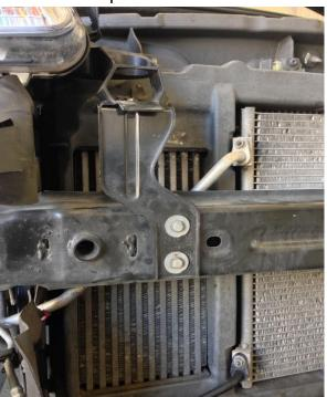
7. Fix intercooler into place with the original bolts
