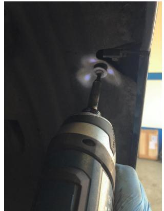
3. Undo 2x 10mm bolts holding bumper to front arch and gently pull the bumper to unclip.
