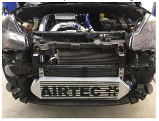
8. Loosely fit in place the pipework making sure the 57mm ends go onto the top engine pipework. Once happy tighten jubilee clips.
