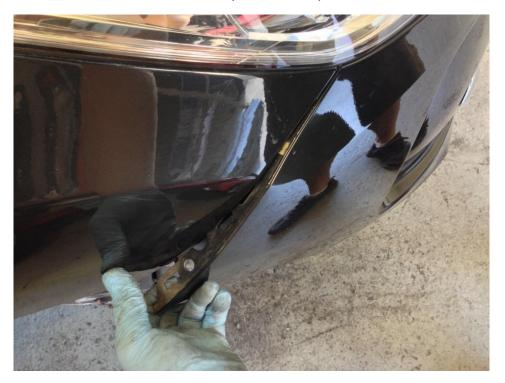
4. Remove bumper making sure to unclip fog lights.
