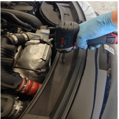
2. Undo T20 Torx and plastic clips securing inner arch to bumper.
