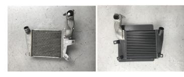
6. Fit new AIRTEC intercooler using original rubber bushes and 13mm nuts
