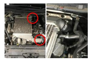
3. Remove 2x 10mm bolts securing standard BOV
