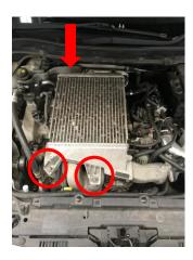
5. With intercooler removed, swap induction elbow including gasket from standard to AIRTEC
