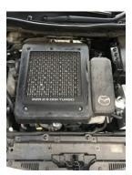
2. Undo both jubilee clips securing boost pipes
