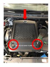
10. Undo 3x 13mm nuts securing standard cooler.
