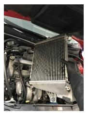
11. Remove N/S & O/S plastic air guides by undoing 2x 10mm bolts
