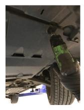
5. Remove 8mm bolt securing bumper to wing
