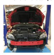
8. Make sure to unclip headlight washer pipe ambient air temp plug and fog lights
