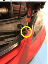
3. Undo 2x plastic screw fittings holding inner arch to bumper and 3x 8mm bolts underneath
