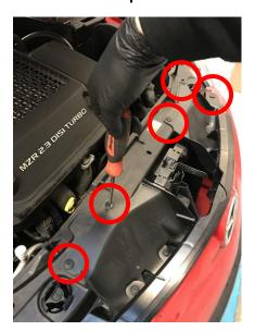
2. Undo 2x Phillips screws holding top of bumper
