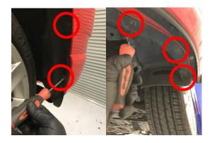
4. Remove engine under tray 7x 10mm bolts + 2x plastic push fit fittings
