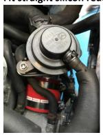
Fit hard pipe with BOV outlet into silicon then 90 degree silicon connects into intercooler
