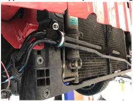
13. Loosely fit intercooler into place and secure with supplied M6 x 20 socket head bolts and washers & M8 by 12 hex head bolts
