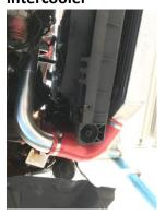
NOTE: Make sure at least 50mm of clearance is left between cold side hard pipe and gear selector arm
