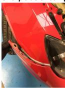
7. Remove front bumper. Please note: the 2 centre clips can be a bit tight to remove
