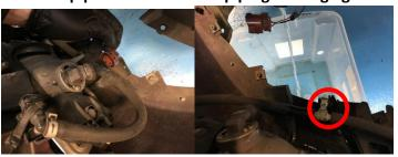
9. Remove standard intercooler cover 3x 10mm bolts to get to standard intercooler
