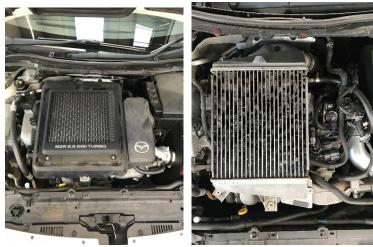
2. Remove standard intercooler by undoing 3x 13mm nuts, BOV 2X 10mm bolts & front + rear boost hoses.
