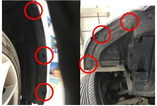
5. Remove 3x 8mm bolts & 2 cross head screws securing bottom of bumper
