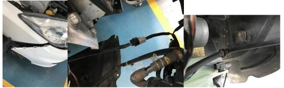
7. Remove standard crash bar by undoing 8x 14mm bolts & 4x 10mm bolts securing radiator housing, 1x 10mm bolt securing centre bar
