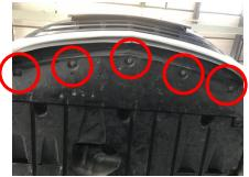
6. Unclip sides of bumper and remove bumper making sure to unclip fog light loom and headlight washers. Store bumper in a safe place to prevent damage.
