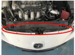
4. Remove 1x 8mm bolt & 3 plastic push fit fittings securing inner arch to bumper, 3x 8mm bolts securing bumper to arch liner
