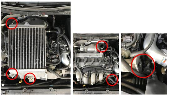
3. Remove 2x 10mm bolts & 6x plastic push fit fittings securing top of bumper
