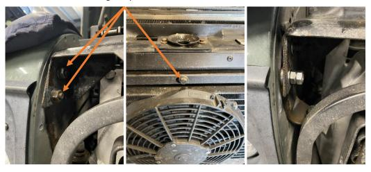
4. At this stage you will need to find a support for the bonnet. Once you have supported the bonnet you can then remove the 4 x 8mm bolts (2 each side) holding the brackets on both sides in place. On the left hand side the top bolt undoes the bracket that supports the air conditioning pipework. This cannot be removed so just slide the bracket up the pipe and out of the way.
