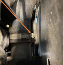
6. Now undo the 2 x 13mm bolts at the top of the intercooler.
