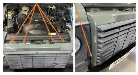
2. Now remove the fan shroud by undoing 6 x Philips screws holding it in, these screws are captive and so will not fully come out.
