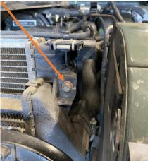
7. In order to remove the intercooler you will need to undo the 2 bolts at the bottom of the air conditioning condenser surround. This allows the surround to be pulled forward slightly whilst a second person lifts up the left hand side of the intercooler, first to release it and then rotate it round slightly before lifting out the right side.
