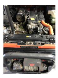
2. Remove the plate on top of the radiator and intercooler by undoing the 4 x 10mm bolt (there is a nut on the underside) and 4 x 13mm bolts. Once undone the surround can be lifted off and out.
