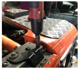
3. Remove hoses attached to original intercooler, you may need to remove a P-clip bolted to the right hand arch in order to remove the original hose from the intercooler.
