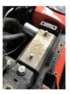
5. Optional step: trim the panel on the right hand side of the intercooler, the intercooler does fit without trimming but is very tight. You only need to remove the front and rear of this panel (see pictures below).
