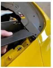
2. Once the side pieces are removed you will be able to access the 10mm bolt at the top of the wing. These will need to be removed from both sides of the car. Then remove another 10mm bolt from both wheel arch liners.
