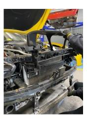
9. You will now need to cut this surround so that your AIRTEC Motorsport intercooler can be installed. Cut the bottom section off as shown in the pictures below.
