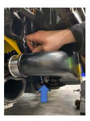
11. After the bottom of the intercooler is secured in place you can fit the new top brackets. You will need to reuse the 13mm bolt removed in Step 5 from the top bracket with the rubber bushings to secure the pins from the intercooler in place.
