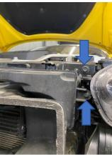
8. Once the air feeds have been removed you can remove the 10mm fixings securing the plastic surround in place. There will be two located at the top of the surround and two above and below the crash bar fixing points, as shown below. After removing the bolts you will need to release the wiring connector that is attached at multiple points using a trim tool. The surround can now be removed.
