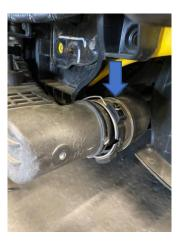
6. Now you will need to remove the lower intercooler brackets by removing two 10mm bolts from either side of the intercooler. The original intercooler can now be removed from the car.
