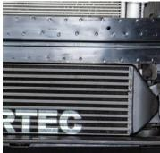
13. Install the provided bracket to the right-hand side of the crash bar with the supplied M6 fixings. Clip the temperature sensor in as pictured.
