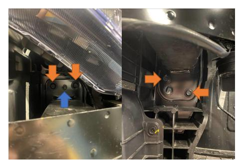
8. Undo the four 10mm bolts (highlighted with orange arrows) holding the air guide to the front of the intercooler. Tilt it forward and then pull upwards to release. This is not reinstalled when reassembling the car.
