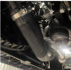
10. To remove the intercooler, undo the four 10mm bolts (highlighted with orange arrows) holding it on and then safely place aside.
