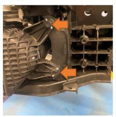
11. Install your new intercooler reusing the fixings that were holding in the original intercooler and fit the new silicone hoses using the supplied jubilee clips and tighten once happy with the fitment.
