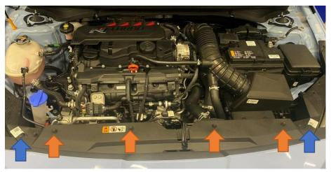
3. Working in the front wheel arches, remove the three trim clips (highlighted with orange arrows) followed by the 8mm bolt (highlighted with blue arrow) that attaches the front bumper to the wing on both sides.
