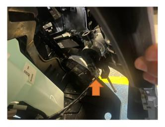
6. Unhook the temperature sensor from the crash bar.
