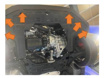
5. With a second person to help, you can now pull the edges of the bumper out to release it whilst one of you holds the bumper the other can undo the fog light plugs on either side.
