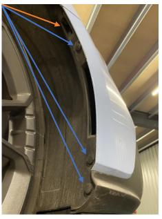
3. There are 6 x plastic clips to be removed along the top of the bumper under the bonnet.
