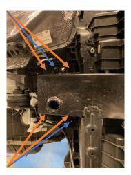
7. Remove the surround by undoing 4 x 10mm bolts and pulling the ducting out of the locating pins, the ducting is not refitted once your new intercooler is installed.
