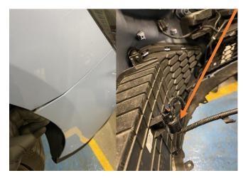
5. Unclip temperature sensor from the crash bar.
