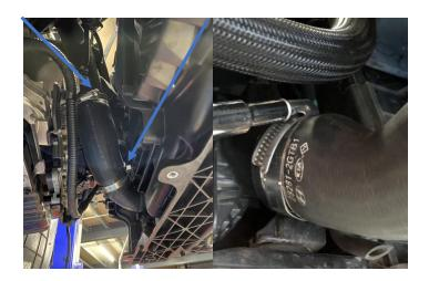
9. Remove the intercooler by undoing the 4 x 10mm bolts and pulling it forward away from the car.
