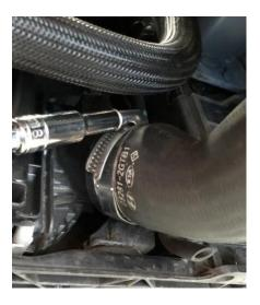
10. Remove the intercooler by undoing the 4 x 10mm bolts and pulling it forward away from the car.
