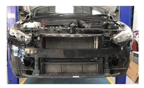
8. Unclip wiring loom from the surround and then remove the surround by undoing 4 x 10mm bolts and pulling the ducting out of the locating pins, the ducting is not refitted with the new intercooler.
