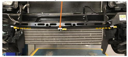
9. You can now install the intercooler to the vehicle. Tilt the intercooler forward and position the bottom pins into the holes before standing the intercooler up. Once upright you can then reinstall the brackets with the original fixings. Unbend and reinstall the crash sensor on the central bracket.
