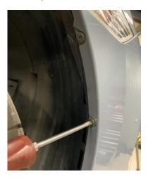
4. Unclip the top of the bumper by releasing the x2 clips above each headlight, to do so you will need to insert a pick tool inside the square gaps and press down until the clip releases.
