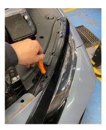
5. The front bumper can now be removed by unplugging the wiring harness connections to the headlights.
