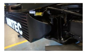
10. Once the AIRTEC intercooler is in place you can install the pro hose pipework which will replace the stock boost pipes. These will need to be secured in place using the supplied jubilee clips.
