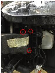
10. Undo 10mm bolt securing right/left side boost pipes.
