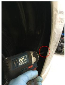
4. Undo 4x T30 bolts along bottom of bumper.
