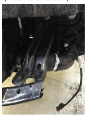
7. Remove 2x 8mm bolts & remove side shields clipped on at top.
