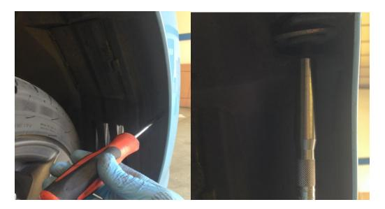
2. Remove X head screws on each side of the inner arch and x 2 torx screws securing the bumper to the wing. As shown above
