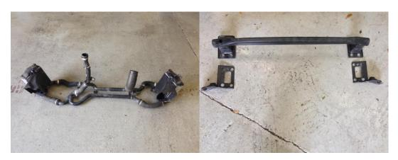
5. Remove all pipe work shown, there is 10mm bolts securing the metal pipework, then remove lower front crash bar and standard intercooler brackets (these will not be replaced)
