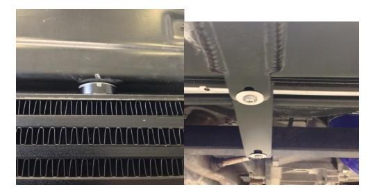
7. Once the intercooler is marked in position remove and drill 2 x 10mm holes to secure intercooler. This can be carried out with top crash bar in place, once secure install lower intercooler support bracket with fixings provided
