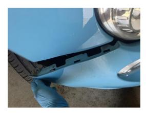
3. Un-clip each side of the bumper and carefully bring forward and un-clip fog light multi-plug
