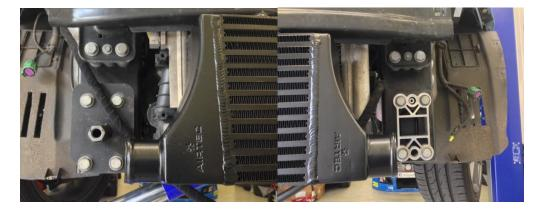
6. Install tow eye bracket as shown, then place intercooler in position as shown, the intercooler should be central to crash bar fixings.
