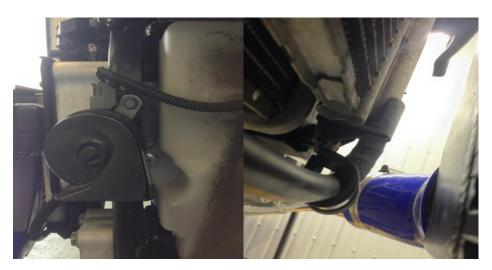
8. Now undo the securing bracket on the horn and move into position as pictured, install 'p' clip around washer pipe as pictured to prevent rubbing
