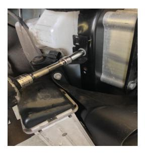
4. Remove the 10mm bolts securing standard intercoolers
