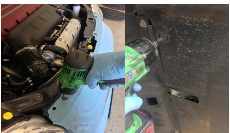
1. Remove x4 torque screws along top of bumper and x 6 torque screws on bottom of bumper
