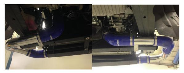
10. The standard under tray cannot be replaced due to the new bigger boost pipes installed. Replace bumper in reverse of removal
