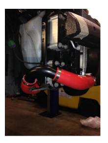
9. Please see layout of pipe work above, all 50mm pipework is on the left hand side and 60mm on the right, loosely install pipework before tightening clip.
