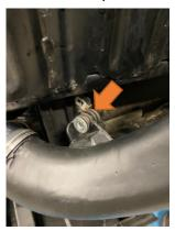
6. Install the new intercooler using the original mounts and 8mm bolts. Fit the supplied plastic push fittings through the upper plastic trim and into the brackets on the sides of the intercooler. Reattach the boost pipes using the original spring clips.
