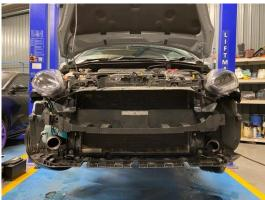
5. Once the intercooler has been removed, you will need to swap the original rubber mounts from underneath the intercooler and the original rubber bushings from the top of the intercooler onto your new AIRTEC Motorsport intercooler.
