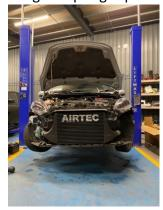
7. Finally, make sure everything has been tightened securely and then reinstall the bumper in reverse of Steps 1 to 3.
