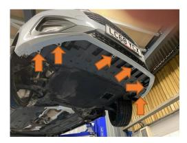
4. Remove the original intercooler by loosening the 8mm bolts securing either side. Then disconnect the boost pipes by levering a flat-bladed screwdriver under the spring clip until you here a 'click'. You can then remove the intercooler from the car.
