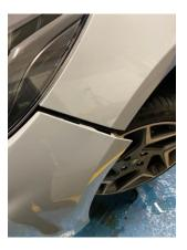
3. Release the six plastic trim clips from underneath the front bumper then unplug the wiring harness and carefully remove the front bumper.
