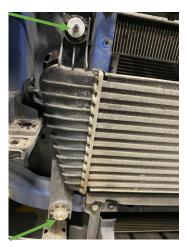
12. Remove the rubber bushes from the original intercooler and fit it to your new intercooler.
