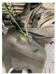
9. Remove the MAP sensor from the intercooler by undoing the T25 torx holding the sensor in.
