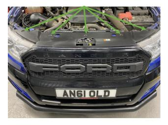
3. Undo the 2 x 10mm bolts that attach the top of the grill to the headlights and then using a long extension undo the 10mm holding the bottom of the grill in on both sides.
