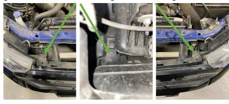
4. Remove lower bull bar if fitted and then under the truck remove the 10mm bolts where the bumper attaches. There are 9 of these.
