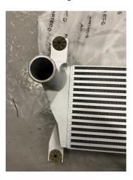
13. Install the intercooler to the truck reusing the original fixings and insert the MAP sensor and tighten using the original torx fixing. Before installing run the temperature sensor down and behind the lower right hand mount off of the intercooler.
