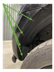
6. Undo the 8mm bolt holding the bumper to the front wing on both sides.
