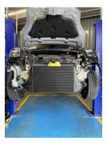
14. Undo the 13mm bolt on each side at the top of the crash bar bracket and install the top intercooler brackets to the car. The shorter of the two brackets goes on the right hand side when looking at the car from the front. Install the M6 x 20mm socket head bolt with penny washer through the bracket and hole in the intercooler and install the second penny washer and nyloc underneath.
