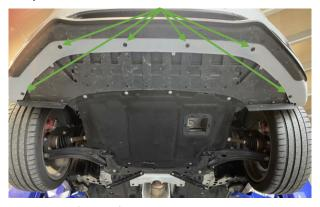
3. The next step is to pull back the front of the arch liners to gain access to the inside of the bumper. You will need to remove the 3 x 10mm bolts along the bottom of each liner and remove 4 x crosshead trim clips by using a cross headed screwdriver to turn them a quarter of a turn and then pull the whole clip out. Once you have removed the clips and bolts then pull the arch liner back and tuck it behind the wheel.
