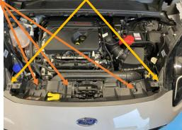
7. With a second person where the bumper meets the arch there is a small clip that will need to be pressed down to release the corner of the bumper. With this released you will be able to pull the edge of the bumper away to release it from the car and then remove the whole bumper. Put aside safely.
