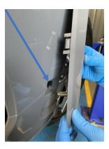
6. Working under the bonnet remove the plastic panel on the right hand side by pulling at the back of it to reveal a 10mm bolt below it. Remove this fitting along with 3 others and 2 x T27 torx fittings. You will then need to unhook the bonnet cable and carefully remove the clip holding the cable to the bonnet latch.
