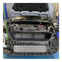
11. The upper surround needs to be removed, to do this you will need to unhook the air temp sensor using a trim tool and then remove the two cross head trim clips by undoing them and then using a trim tool to remove. There are clips holding the bottom of it to the top of the crash bar, starting at one end push down on the clips whilst pulling at the surround to remove. Put aside, this is not reused.
