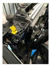
17. The bonnet will now need to be supported via a different method as the bonnet strut is removed with the surround.
