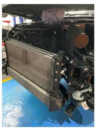
18. Unclip the intercooler pipework and remove the intercooler by squeezing the 2 clips at the top and the intercooler will swing forward and down.
