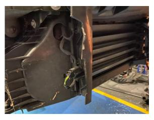
8. Remove 4 x trim clips along the top of the upper surround then squeeze clips either side to release the surround.
