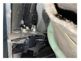
5. Release the bumper from the wing brackets by pulling away from the car.
