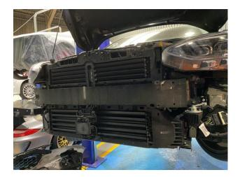
11. Unclip the radar wiring harness then remove the radar by undoing the 2 x T27 screws then lift the radar to remove.
