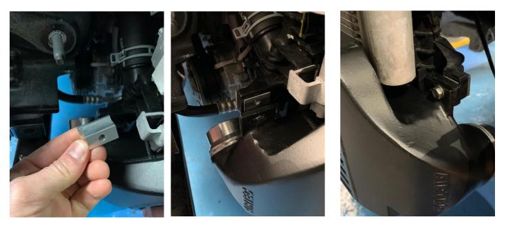
20. The next step is to refit the intercooler / Rad pack casing before fitting you will need to remove the lower flaps and cut plastic to allow the Intercooler fit.
