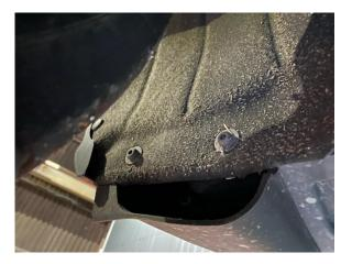
3. Remove 6 x 10mm bolts along the top of the bumper, plus the 2 trim clips and 2 x T27 Torx screws.
