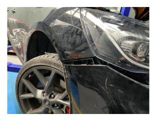
6. Now unclip the wiring harness from inside the driver's side arch liner and unclip 2 harness clips.
