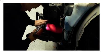
7. Remove 2x 8mm bolts from intercooler under tray to remove intercooler.
