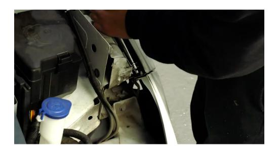
5. Unplug fog lights from front bumper and carefully remove bumper.
