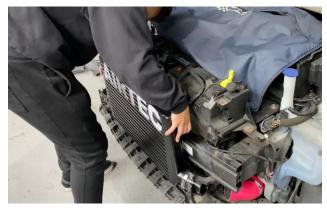
10. You will now need to use the pipe bends provided with the kit to complete the installation of this intercooler. Simply slide them into your boost pipes then attach them to the silicone pipe on your new cooler using the provided jubilee clips (make sure to tighten clips correctly in case of boost leaks).
