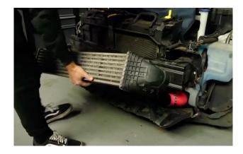
8. Attach 2x silicone pipe using jubilee clips provided.
