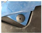
5. On top of the slam panel where the torx fittings where there is a plastic clip, this needs to be pushed up to release the clip and allow the top of the bumper to come forward, then using a second person starting from the edges of the bumper pull outwards to release the corners, unplug the wiring for the fog lights and then proceed to remove the bumper by pulling it out forwards and then store the bumper safely.
