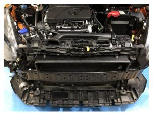
14. The air temperature sensor can now be reinstalled by pushing it into the holes on the new air guide. The wiring for this is best routed behind the new air guide.
