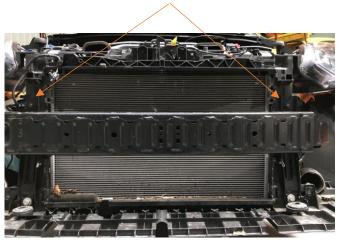
13. Install the new air guide into place where the upper plastic surround was and use the supplied M6 x 16mm socket head bolts with washers and nuts to secure the 2 smaller brackets to the top of the new air guide and reuse 2 of the original push fittings to secure this to the car. (please note that this will be sandwiched between the radiator and intercooler which will help to hold this secure)
