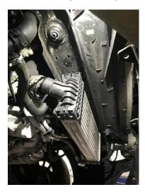
3. Secure radiator and undo 4x 10mm bolts securing radiator and intercooler cradle and remove cradle
