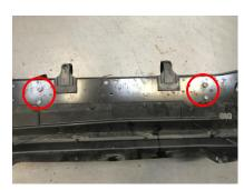
5. Bolt new intercooler into place using original fixing bolts
