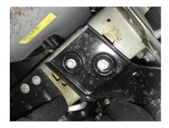
4. Undo 4x T27 torx securing intercooler
