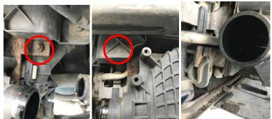
7. Line up AIRTEC intercooler fixing bracket holes with pre-drilled holes on crash bar and loosely bolt into place with supplied bolts
