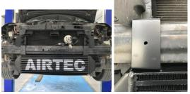
8. Cut radiator cradle front fixings to allow clearance for new boost pipes and fit as pictured.
