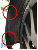
4. Remove 3 x 10mm bolts securing bumper to wing
