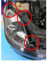
3. Remove 2x T25 torx securing inner arch to bumper
