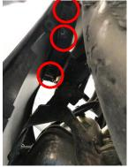
5. Unclip sides of bumper and remove. Making sure to unclip fog lights
