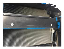
13. Fix intercooler in place with supplied bolts
