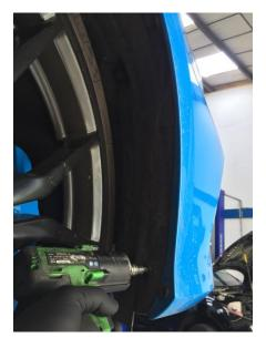
5. Remove plastic fixing clip holding bumper to arch
