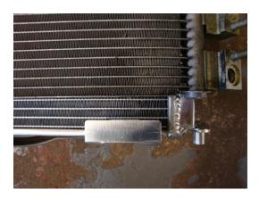
4. Now fit the top securing brackets, start with the left hand side bracket, it has a custom made rubber grommet that slides over the Air-con re-gassing pipe, this secures the Air-con radiator into position
