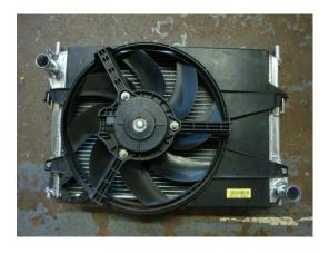
3. Do not remove <u>Air-con</u>, pictures are for instruction only, Hook the lower part of the Air-con radiator onto the Alloy brackets, as shown below.
