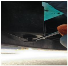
4. Undo the 3 x 10mm bolts securing wing to the bumper (3x bolts each side)
