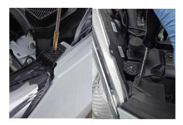
3. Undo  $4 \times T30$  Torx bolts along inner wheel arch liner each side and then remove 2 push fittings along bottom of bumper
