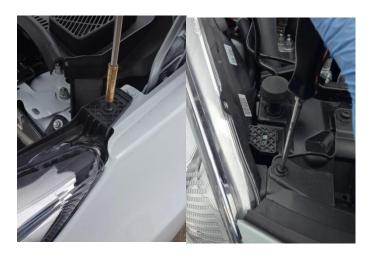
3. Undo  $4 \times T30$  Torx bolts along inner wheel arch liner each side and then remove 2 push fittings along bottom of bumper
