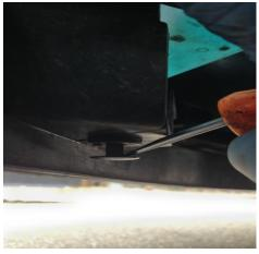
4. Undo the 3 x 10mm bolts securing wing to the bumper (3x bolts each side)
