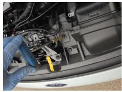
2. Undo  $2 \times T30$  torx bolts on each headlight and remove headlight giving enough room to unclip the multi plug which is located at the bottom
