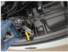
2. Undo  $2 \times T30$  torx bolts on each headlight and remove headlight giving enough room to unclip the multi plug which is located at the bottom
