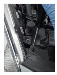
3. Undo 4 x T30 Torx bolts along inner wheel arch liner each side and then remove 2 push fittings along bottom of bumper
