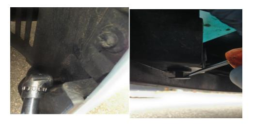
4. Undo the 3 x 10mm bolts securing wing to the bumper (3x bolts each side)
