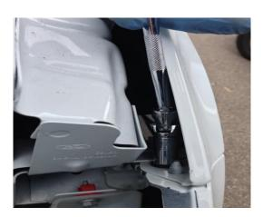
5. With bumper removed you will now need to remove the standard intercooler, undo the 4 crash bar bolts on the left hand side and loosen the right hand bolts, this will then give you access to the intercooler securing bolts, loosen jubilee clip on boost pipes and then remove intercooler. (tip. Mark position of crash bar with marker pen, this will save time aligning it back up)
