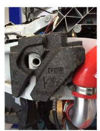
16. Remove air deflector motor, unclip securing tab and securing insert. Remove motor and secure to radiator cradle.
