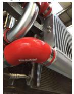
14. Install boost pipes and shown in photo (Fitted photo and product image)
