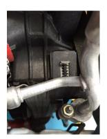
11. Lower radiator cradle, remove x2 10mm left hand side, pull downwards, remove boost pipes and remove stock intercooler
