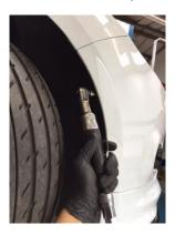
5. Remove torque bolts & push fittings securing under tray
