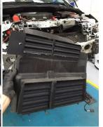
10. Remove OEM intercooler scoop, un-clip and pull downwards then unclip AC pipe from stock intercooler
