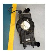
12. Bolt new Airtec intercooler into position with fixings provided, the side bracket fixing can be tightened by gaining access at the end of the crash bar
