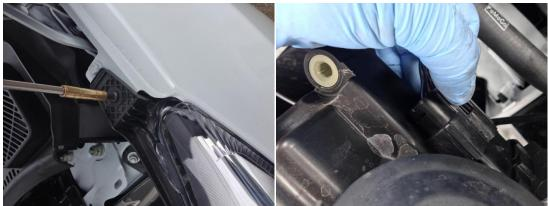
3. Undo 4 x T30 Torx bolts along inner wheel arch liner each side
