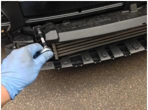
8. Remove the 2 x 8mm bolts holding intercooler, loosen jubilee clips on boost pipes and then the intercooler can be removed.
