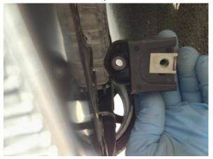
10. Swap over rubber grommet that are located on top of standard intercooler
