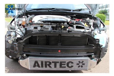
1. Undo 2 x T30 Torque bolts and 4 cross hex plastic screws
