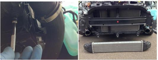
9. Remove lower support bracket, this is no longer required and can be kept if car goes back to standard or thrown away.
