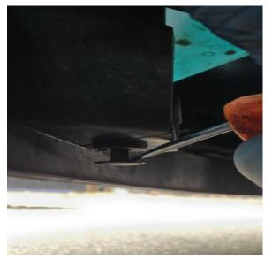
5. Undo the 3 x 10mm bolts securing wing to the bumper (3x bolts each side)
