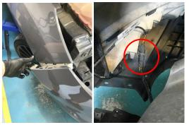
8. Unbolt 2x bolts holding front grill shutters in place
