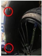
4. Remove plastic push fit fitting securing bumper to wing
