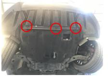
6. Remove 2x plastic push fittings on side of under tray and remove under tray
