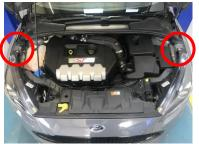
2. Unclip plastic push fit fittings securing bumper
