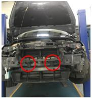
9. Disconnect stepper motor multi plug on side of original intercooler
