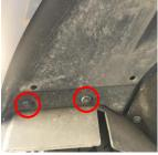
7. Unclip sides of bumper and disconnect multi plug situated behind the bumper, and remove bumper.
