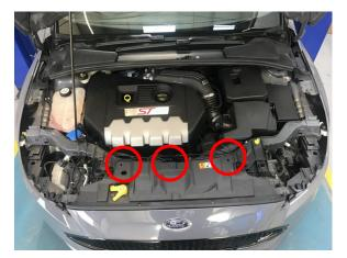
3. Remove 2x Torx bolts securing inner arch to bumper
