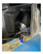
10. Drill out x6 rivets holding the intercooler brace in place, you can then unclip the intercooler tabs and lower down the intercooler and brace then remove.
