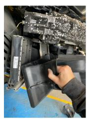
7. Now you will have access to the brake cooling guides, start by removing the T25 Torx screw then slide the guide up and unclip the guide to be able to remove as this will need to be removed in two separate pieces.
