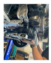
11. You can now remove the stock intercooler and remove the intercooler tab insert as these will not be re used.
