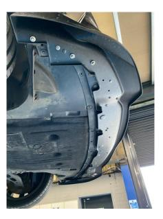
2. Remove the front half of the arch liner out by removing the 8mm bolts holding the arch liner in place as this will make it much easier to access the x2 8mm bolts securing bumper to the wing.
