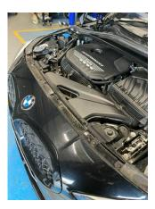
4. You can now remove the front bumper but before removal make sure to disconnect the wiring harness and sensors.
