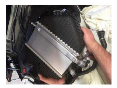
7. Swap the securing brackets onto your new AIRTEC charge cooler with new supplied bolts and reinstall in reversal of dismantling.
