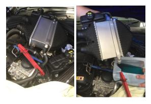
5. Remove the coolant reservoir bottle which is located on the side of the charge cooler, remove the x 2 torque screws and coolant hose then pull the bottle upwards to remove.
