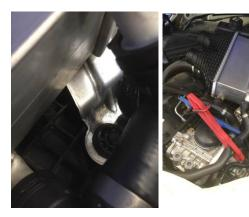
4. You now need remove the coolant hoses that are attached to the charge cooler, you need to keep as much of the coolant as possible, we suggest clamping the coolant hoses and have a container ready to catch the coolant.
