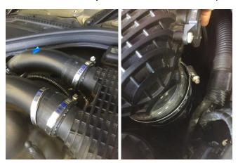
3. The charge cooler is secured with rubber grommets that are located underneath the charge cooler, pull the charge cooler upwards firmly, at the same time the boost pipes and throttle body hose can be removed.
