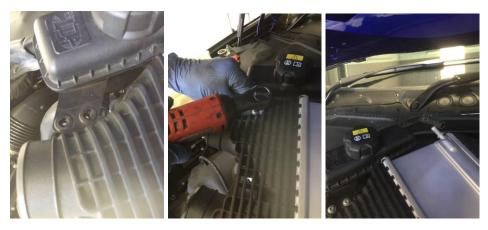
6. You can now remove the oem charge cooler, place it upside down on a flat surface
