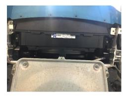
7. Once in position, clip original boost pipes back onto the intercooler and secure intercooler using the stock bolts, fit under tray back on.
