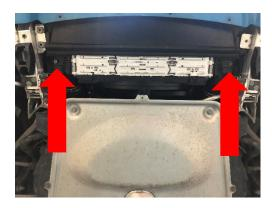
5. Carefully pull down the plastic air guide (this is flexible, be careful not to break). Tilt the intercooler towards the front of the car and carefully remove, making sure the boost pipes aren't attached.
