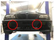
4. Unclip sides of bumper and remove bumper making sure to unclip fog lights
