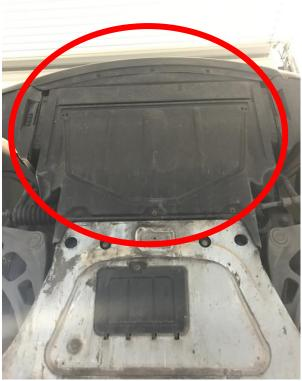
2. Undo 2x8mm bolts holding inner arch to bottom of bumper
