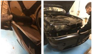
5. Remove both brake air guides 2x8mm bolts
