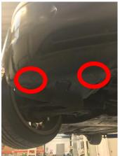
3. Undo 2x main bumper fixing bolts E12 torx located under headlight section of bumper
