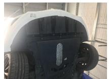
6. Unplug bumper loom and remove bumper
