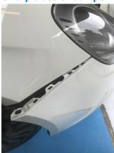
5. Remove 18x T27 torx and 3x crosshead screws securing front lower under tray
