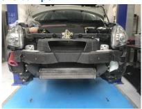
7. Remove standard intercooler by removing 8mm bolt securing plastic air guide, remove boost pipes, unclip cooler and remove. Trim lower plastic air guide as pictured
