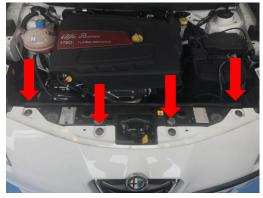
2. Remove T27 torx securing bumper to wing
