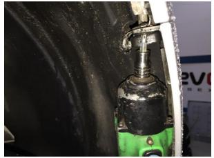
3. Undo 3x Phillip screws on sided of bumper (1x located underside of bumper).
