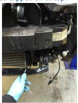
If you cannot remove, cut lower sections to allow intercooler fitting.
