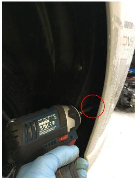
4. Undo 4x T30 bolts along bottom of bumper.
