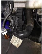
13. If you wish you can remove/ cut off securing brackets on boost pipes as these are no longer needed.
