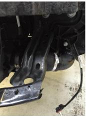
7. Remove 2x 8mm bolts & remove side shields clipped on at top.
