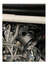
13. Before installing the enclosed intake, you will need to fit the stick on foam piece to stop the paintwork being damaged as seen in picture below.
