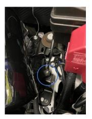
15. Now reinstall the MAF sensor using the provided M4 x 8mm button head bolts then check everything is in place and tightened correctly.
