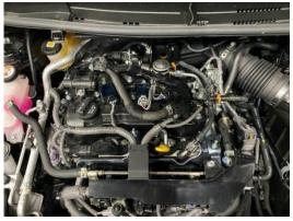
3. Unplug the solenoid and unclip vac line from the front of the airbox then continue to unclip the vac line back to the T-piece on top of the inlet pipe and then remove.
