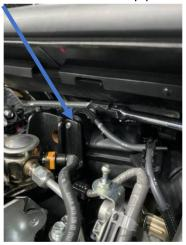
10. Install new inlet pipe using 1 of the original 12mm bolts. Leave the jubilee clip loose for now.
