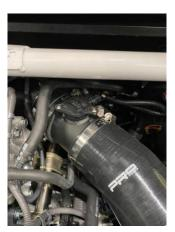
16. Install silicone bung for VAC line. The vac line can be tucked down and secured with a cable tie.
