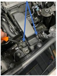
6. Loosen the 10mm hose clip attaching the airbox to the inlet pipe.
