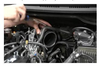
12. Now the silicone coupler is secured in place you can install the MAF sensor pipework.
