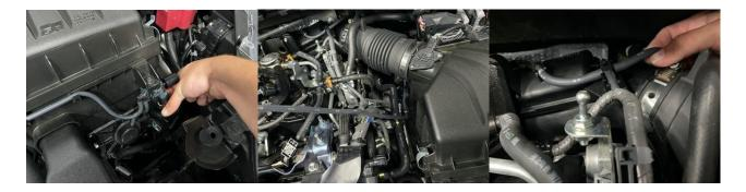
4. Unplug the MAF sensor and unclip the harness from the top of the airbox using a trim removal tool.
