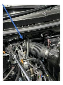
7. Pull the airbox up and to the left so that you can access the wiring for the solenoid, remove using a trim removal tool and then pull the airbox up and remove from the car. (Tuck the solenoid wiring on the right handside and secure using a cable tie or similar)
