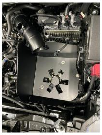
14. Install your new MAF pipe and use supplied M6 bolt and washer to attach the bracket to the pipe.
