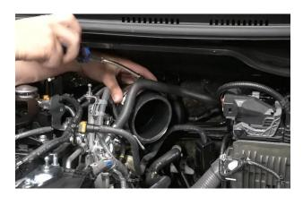
13. Install your new induction shield making sure to push the pins firmly into place. Install using supplied M6 bolts and washers (Shortest pin at the back, medium in the middle and longest at the front.)
