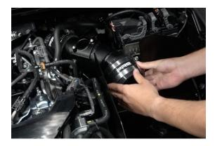
15. Install the silicone coupler and install filter. Position filter to ensure there is no rubbing against the shield
