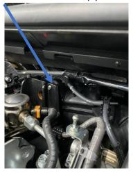
10. Install new inlet pipe using 1 of the original 12mm bolts. Leave the jubilee clip loose for now.
