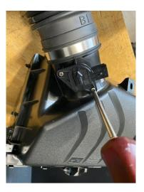
18. Install silicone bung for VAC line. The vac line can be tucked down and secured with a cable tie.
