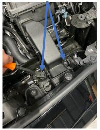
6. Loosen the 10mm hose clip attaching the airbox to the inlet pipe.
