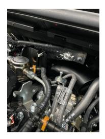
11. Remove 12mm bolt and install supplied bracket.
