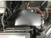
6. Fit vacuum pipe + supplied bracket to AIRTEC intake pipe, loosely bolt to induction shield with supplied nuts and bolts
