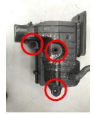
5. Locate new induction shield into place and bolt to battery tray using supplied M6 X 50 socket head & mudguard washer
