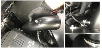
7. Fit AIRTEC air filter to induction pipe.
