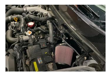
11. Lastly re install the OEM air guide and check that everything has been tightened correctly and is secure.
