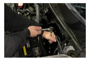
9. Reinstall MAF sensor using the supplied M4 fixings and reinstall the vac line.
