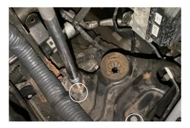
8. Install your new AIRTEC heat shield by lining the two holes in the bottom of the shield in line with the holes from the bolts you just removed and then install the provided M8 fixings to secure the heatshield.
