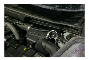
2. Now unclip the MAF sensor wiring harness from the stock airbox.
