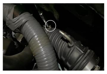
6. Start installing your new AIRTEC intake by fitting the silicone hose to your new induction pipe using a jubilee clip to secure.
