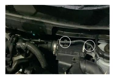
3. Remove the x2 7mm MAF sensor bolts then carefully remove the sensor.
