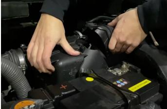
5. Using pliers remove the vac line by applying pressure on the clip then sliding it off, you can now remove this induction pipe by loosening the jubilee clip with a jubilee flexidriver or 7mm socket.
