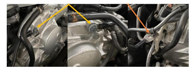
9. Undo the two 12mm bolts holding on each dump valve to the top intake tubes and move them out the way. (The hoses can remain connected and just locate them away from the airbox to make it easier to get the boxes out and new pipes in.) Pull the gasket off and keep safe.
