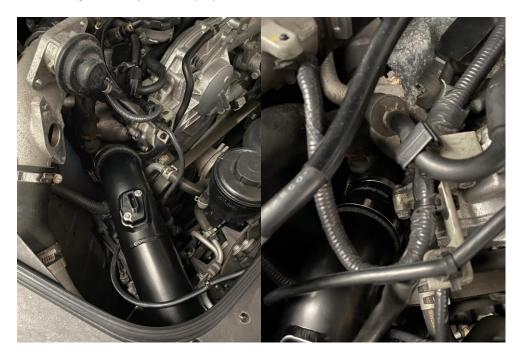
18. Get the supplied bracket and place it on to the bolt that you inserted earlier and then use the washer and nyloc to secure. Line up the other two holes on the bracket with the two threaded holes on the machined block on top of the induction pipes and once happy with the position insert 2 x M6 bolts with washers in to each side and tighten.
