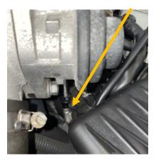
8. Undo the ends of the earth strap on both sides of the cylinder head by removing the 12mm bolt holding it in and unclip the wire from the brackets allowing the earth straps to be moved out of the way.
