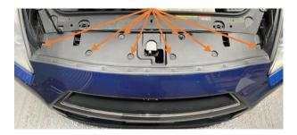
3. Remove the plastic trumpet each side by removing the plastic clip holding it on.
