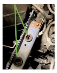
11. Unclip the earth strap from the bracket holding it down to the chassis along with removing the wiring loom by pushing in on the back of the tab and wiggling the holder off, once removed then undo the 12mm bolt and remove the bracket from each side.
