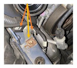
12. Undo the jubilee clips (8mm) holding the hose on to the turbo and remove the hoses. Take care not to drop anything into the turbo inlet.
