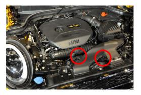
2. Unplug MAF sensor and also unclip breather pipe
