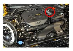
3. Remove standard airbox and induction hose, airbox is held in by 1x 10mm bolt securing to inner wing and 2 push fit fittings
