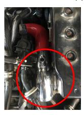
6. Fit supplied induction shield, securing the back of the shield to existing M6 stud and front of shield using supplied bracket
