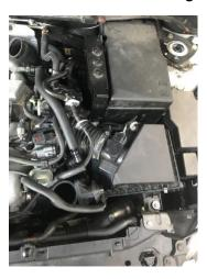
2. Remove standard induction pipe secured by 1x 10mm nut. Please note this is a tight fit to get out.
