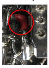
5. Fit intake hard pipe to silicone 90
