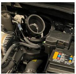
6. Undo the 10mm bolt highlighted and place the induction pipe bracket over the hole and reinstall the bolt, but do not fully tighten yet to allow movement.
