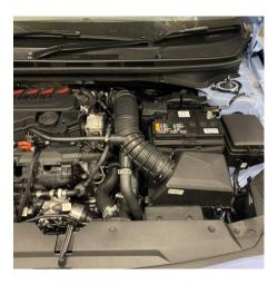
2. Undo the two hose clamps highlighted below using the pliers and then disconnect the hoses.
