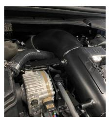
8. Next, fit the new wiring harness bracket using the original 10mm bolt located in the front panel, as shown. Use the bracket to attach the wiring loom clip disconnected in Step 4.
