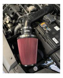
12. Once happy with the overall fitment and alignment of everything, fully tighten the rear jubilee clips and the bolts holding the bracket in place.
