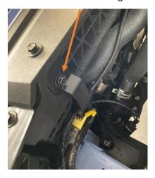
9. Now assemble the heat shield using the M5 nuts, bolts and washers supplied, as shown.
