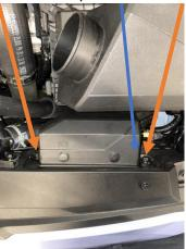
5. With the air box removed you can now begin installing the replacement induction pipe. Firstly, install the silicone reducer onto the turbo elbow with the 70mm jubilee clip supplied.
