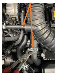
3. Undo the two 10mm hose clips highlighted and remove from the car.
