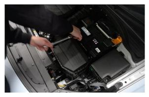
2. Once the airbox has been removed loosen the jubilee clip securing the intake pipe to the airbox by using a 10mm socket on your ratchet.
