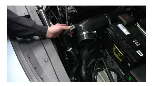
11. Finally reinstall the airbox and air feed in reverse of removal then check that all jubilee clips and fittings have been secured correctly.
