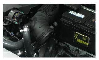
3. You will now need to remove the stock Symposer hose which will be connected to your lower boost pipe and intake hose. Release and remove the hose by squeezing the clips with a pair of pliers.
