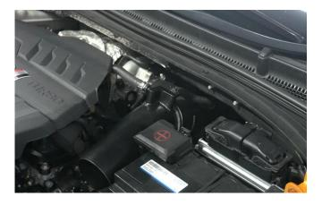
9. Now install your last silicone joiner which will attach from the alloy pipework to the airbox. There is also another connection on this pipe work that will attach the Symposer for this pipework to connect you will need to instal the alloy joiner at the connection as showed in the image below.
