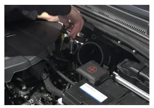
8. After installing the silicone elbow you will need to install the alloy pipework part of this induction kit. Slide the pipework into the elbow and secure with provided jubilee clips. You will also need to now re-attach the x2 breather hoses.
