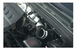
5. Now you will need to remove the stock turbo elbow which is bolted to the turbo elbow using x3 10mm bolts. Once these have been removed the elbow can be removed but make sure to not lose the gasket which will be attached to the end of the gasket. You will also need to detach the wiring that has been clipped onto the underneath of the turbo elbow.
